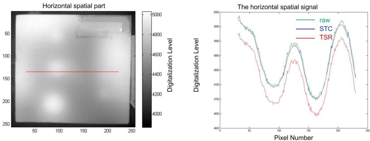
**Fig. 3.** : Left: Selected frame no. 300 from the cooling sequence. Right: horizontal signal line profile along the marked line for the three cases raw, STC and TSR.
