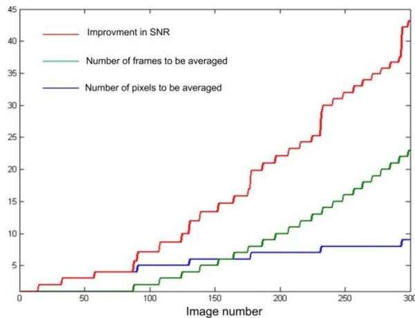
**Fig. 2.** : Spatial and temporal averaging and calculated improvement of SNR in a metal sample as a function of the frame number
