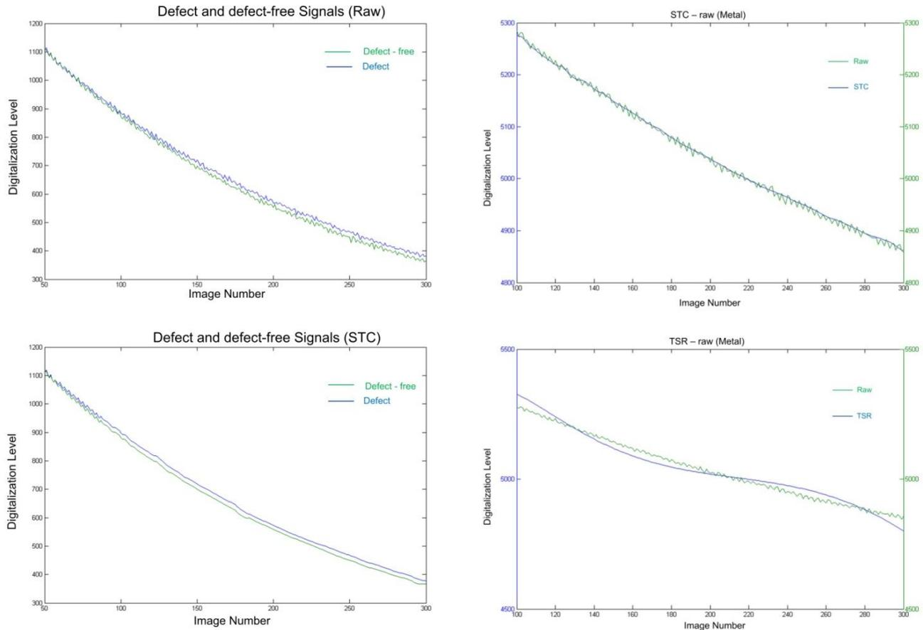
**Fig. 4:** Left: (Top) Defect and defect-free signal of the raw data (top) and after STC filtering (bottom). Right: Comparison between the raw data and the STC (top) and the TSR (bottom) temporal signal
